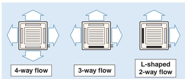
\*For 3-way or 2-way flow installation, the sealing member for air discharge outlet (option) must be used to close each unused outlet.
