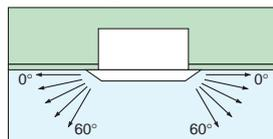
\*Angles can be also set on site to prevent drafts (0°-35°) or soiling of the ceiling (25°-60°), other than standard setting (0°-60°).
